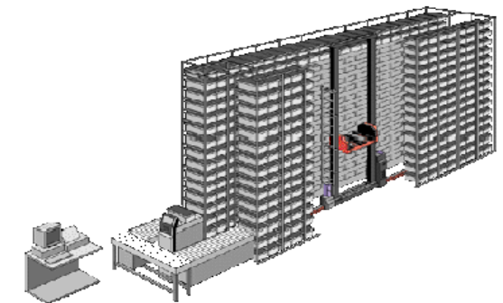
Fully automated small-parts warehouse „Miniload warehouse“
