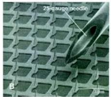
Fig. 1. (A) Schematic representation of the Macroflux\* microprojection array integrated with an adhesive patch. (B) Scanning electron photomicrograph of an array of microprojections (330 µm length). For scale, a 25-gauge needle is shown adjacent to the array.
